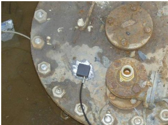
Figure 2.9: SMS Adhered to Flange
